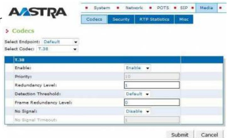
The screenshot shows the Aastra web interface with the 'Media' tab selected. Under 'Codecs', the 'T.38' configuration is visible. The 'Redundancy Level' is set to 1. Other settings include 'Enable' (checked), 'Priority' (10), 'Detection Threshold' (Default), 'Frame Redundancy Level' (0), and 'No Signal' (Disable).
